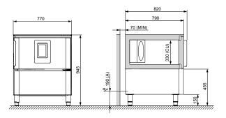
(M1) MX20ATS7(M2) SXP 7 A TS7(A) Electrical power supply(CU) Useful(MIN) Minimum
