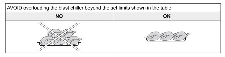
Do not place the trays too close to each other so as to avoid uneven air circulation inside the blast chiller
