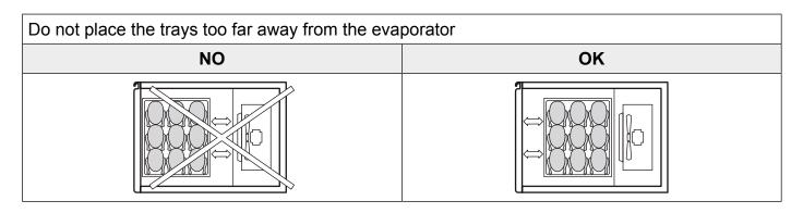
Do not concentrate the trays in one area of the blast chiller in case the load is not complete; distribute its height evenly
