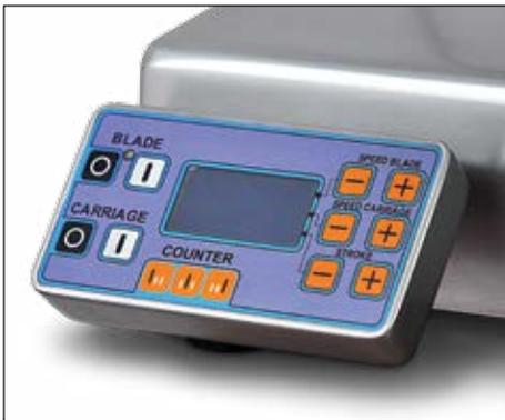
Electronic control panel for automatic operation.
