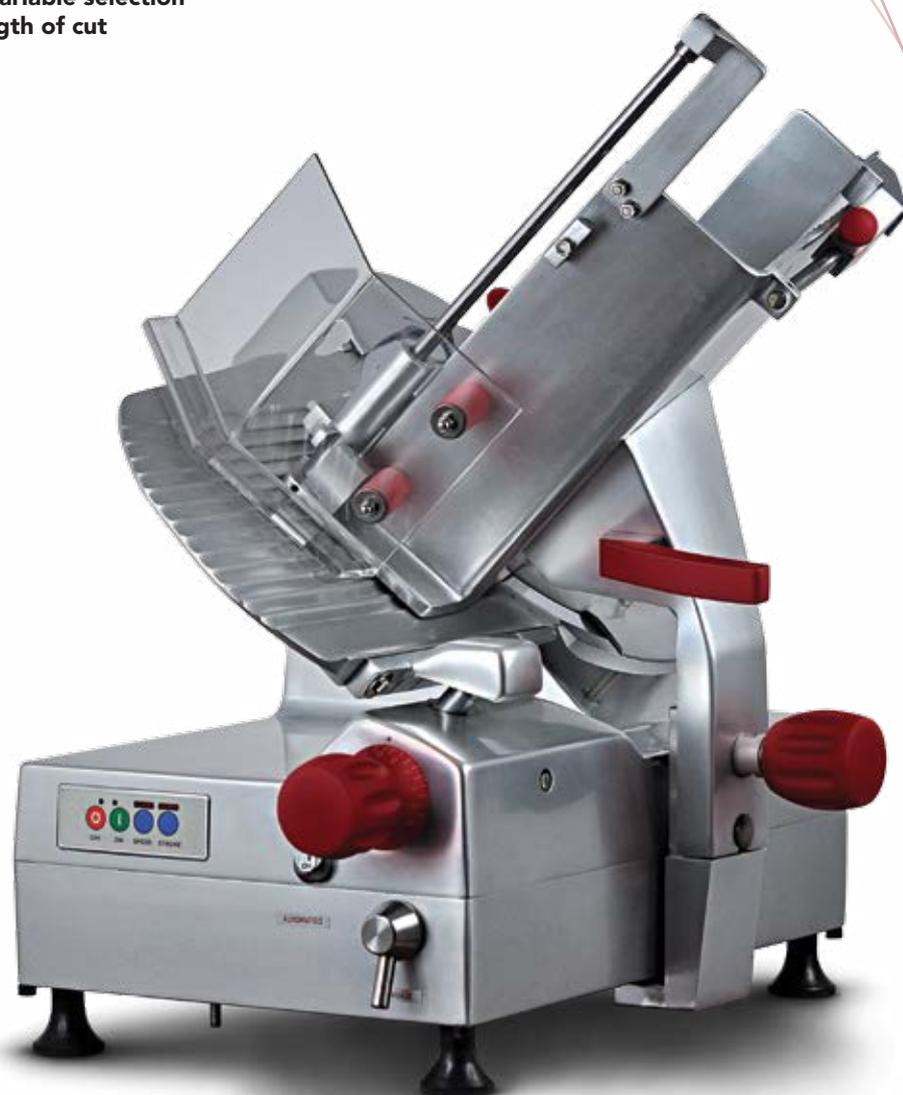
The semi-automatic gravity feed belt driven slicer is designed for volume cutting and features two independent motors, one for blade rotation and the other for carriage movement. The slicer can be used either manually or with automatic operation. In the automatic mode, 3 carriage movement lengths can be selected to suit the size of the product and three carriage speeds can be selected to suit the delicacy of food being sliced.
