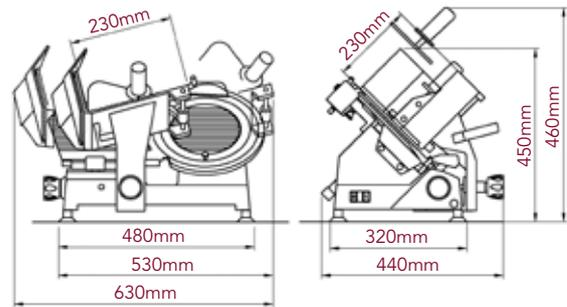
**Manual Gravity Feed Gear Driven Slicer - Heavy Duty**
