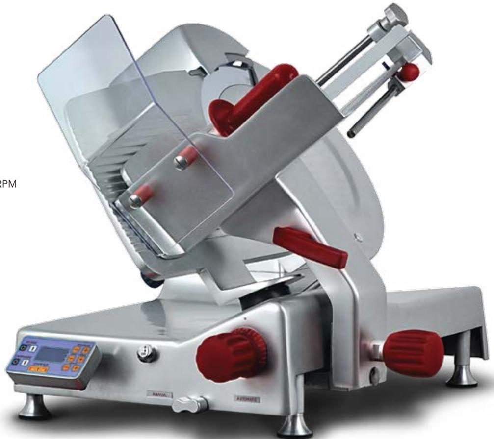
The fully automatic gravity feed belt driven slicer takes the hard work out of slicing. It is fast, clean, precise and very easy to operate and features two independent motors, one for blade rotation and the other for carriage movement.
