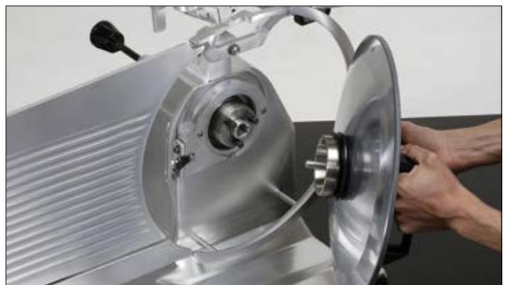
Premium model NS350HDX is available with factory fitted speedy blade remover guard.
