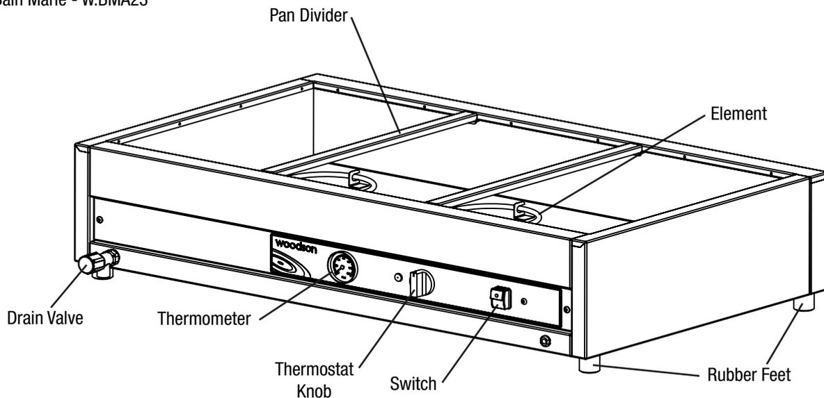
These bain maries may be used wet or dry, depending on the application. Once unit has been used as a WET bain marie it cannot be used dry as the elements will have absorbed moisture and water borne minerals which will affect the reliability of the unit should it be run dry.
